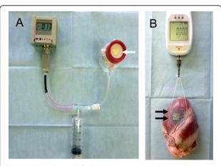
**Figure 1 Experimental design. A:** Experiment 1; An airtight circuit is formed from a pressure gauge, a plastic syringe, and a pressure-hardened plastic tank covered by rabbit skin with 5 holes. The holes are covered with TachoComb sheets (arrow). **B:** Experiment 2; A silk suture loop was placed on the pericardium and fixed with a TachoComb sheet plus a PGA sheet and fibrin glue (arrows). After stabilization, tension was gradually applied to the loop with a digital gauge.
