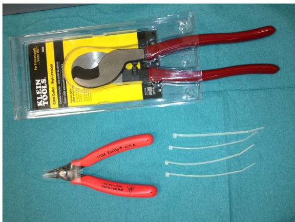
Figure 2 Set of tools: Xcelite 170 M general purpose shear cutter (Apex tool group, Sparks, MD, USA), high leverage cable cutter (Klein Tools, Lincolnshire, IL, USA), cable ties.
