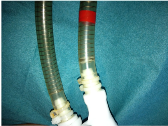
Figure 1 Small horizontal tear at the left ventricular driveline.
