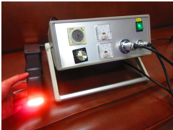
Fig. 1 Infrared coagulator "Kyo-co". The cuboid quartz rod exit plane has a rectangular (30 mm × 10 mm) surface designed to enable creation of a linear lesion. Light from a tungsten-halogen lamp emerges as 35 W/cm 2 of near-infrared light energy (wavelength: 400 to approximately 1600 nm; peak wavelength: 850 nm)
